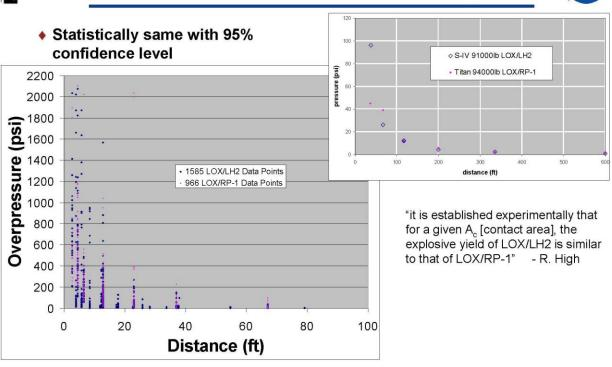
This allows limited accident data to be statistically relevant for both LOX/RP and LOX/LH2
