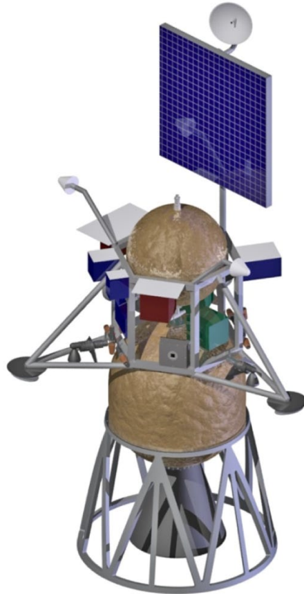
Figure 1.1—Robotic Lunar Lander shown on top of Star 27 solid rocket motor.
