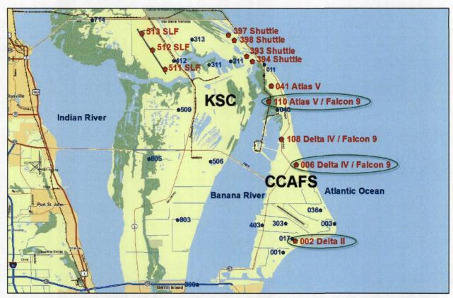
Figure 9. Map of KSC/CCAFS showing the locations of the wind towers used to verify MesoNAM forecasts (red pentagons labeled with tower number and the supported launch activity) and the dual-sensor towers (green ellipses). The onshore and offshore stratifications were determined by the coastline alignment relative to the Atlantic Ocean for each tower.
