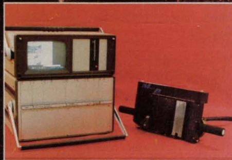
MAUS Provides fast, in-place inspection of composite parts.
