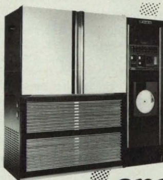
Figure 1. The Achromatical Optical Correlator uses multiple-pinhole diffraction of dispersed white light to form superposed multiple correlations of the input and reference images in the output plane.
