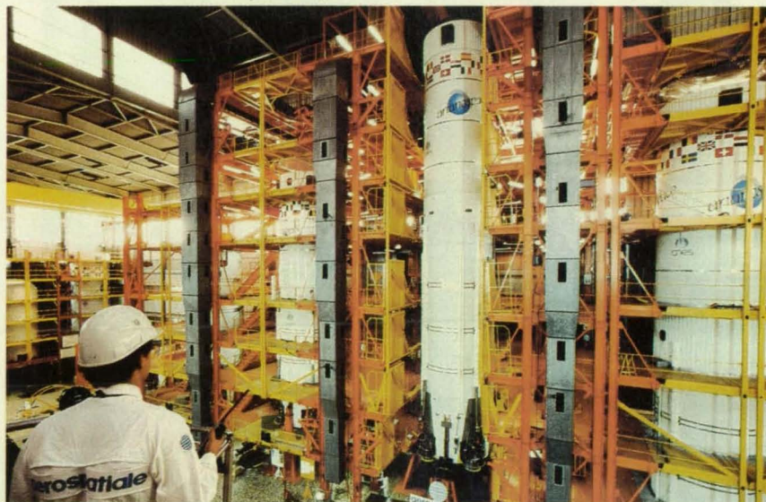
Aerospatiale assembles the first and third stages of the Ariane 4 at its integration and testing facility in Les Mureaux, near Paris.
