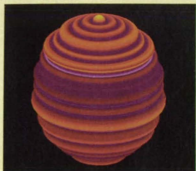
The initial stages of solidification of a small solid nucleus are traced in time, showing the natural development of solid-melt interfacial instabilities. These instabilities later result in tree-like dendritic structures common in many types of solidification.
