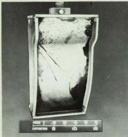
ORIGINAL CONTOUR AFTER 105 HOURS OF ELECTROFORMING, SHOWING SOME NODULES
