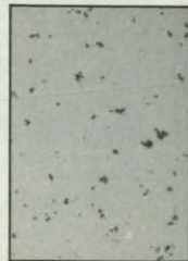
Photomicrograph shows microshrinkage in as-cast condition A356 aluminum. Magnification: 3x
