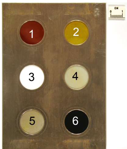
Figure 3. Sample holder with six polymer samples.
