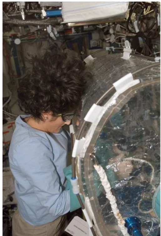
Figure 3.—Astronaut Sunita Williams conducts a soldering experiment within the MWA Containment System aboard the ISS.
