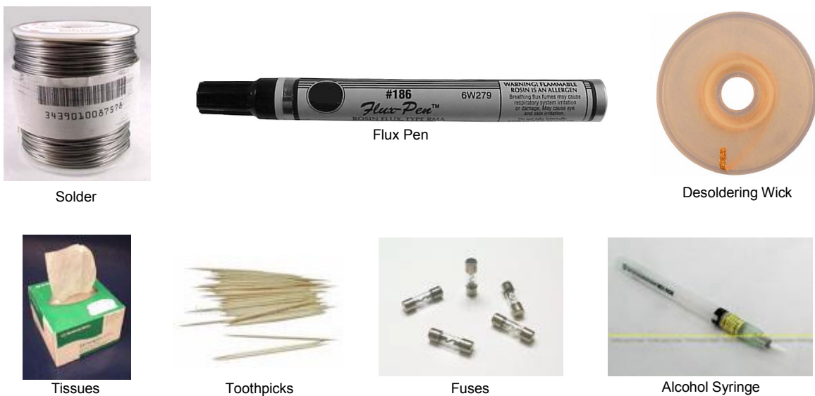
Figure 7.—Images of recommended materials and supplies to allow for component-level repair of electronics. (Note that images are not to scale.)
