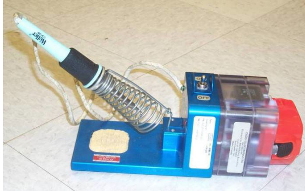
Figure 2.—Soldering iron from the US Soldering Kit, used on the ISS.
