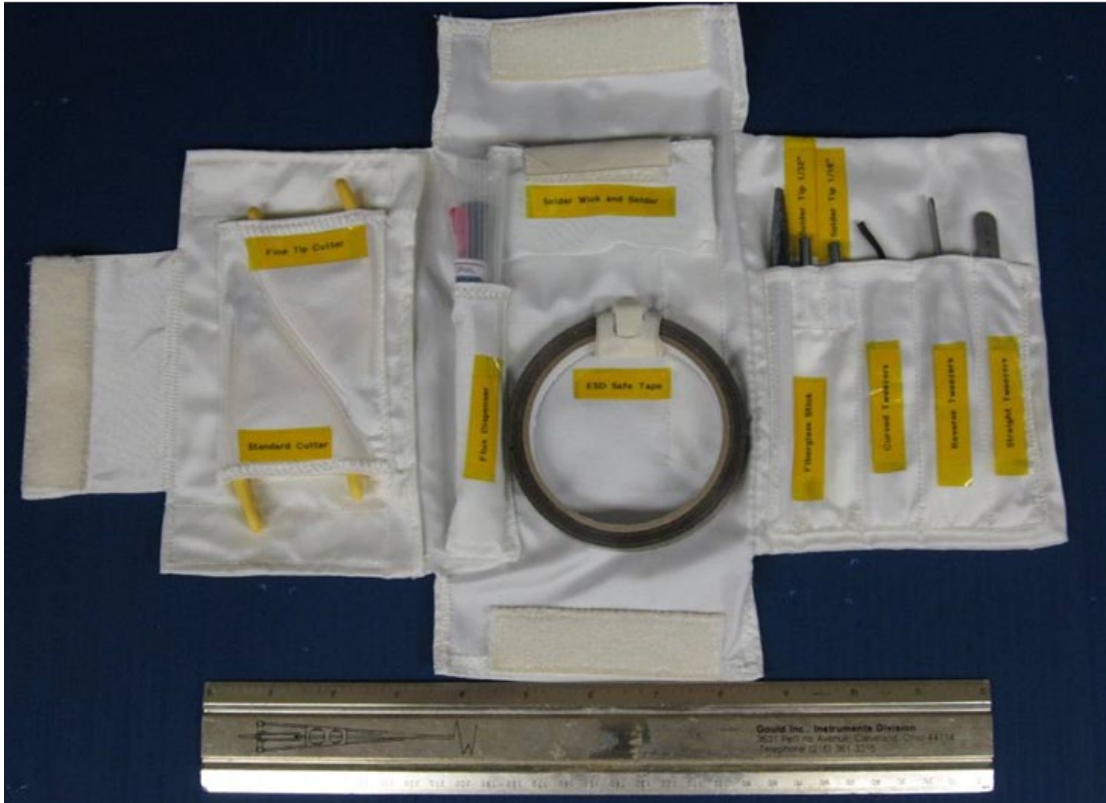
Figure 9.—A set of small tools, used for electronics repair, sent to the ISS as part of the CRE-1 experiment which operated in 2009.
