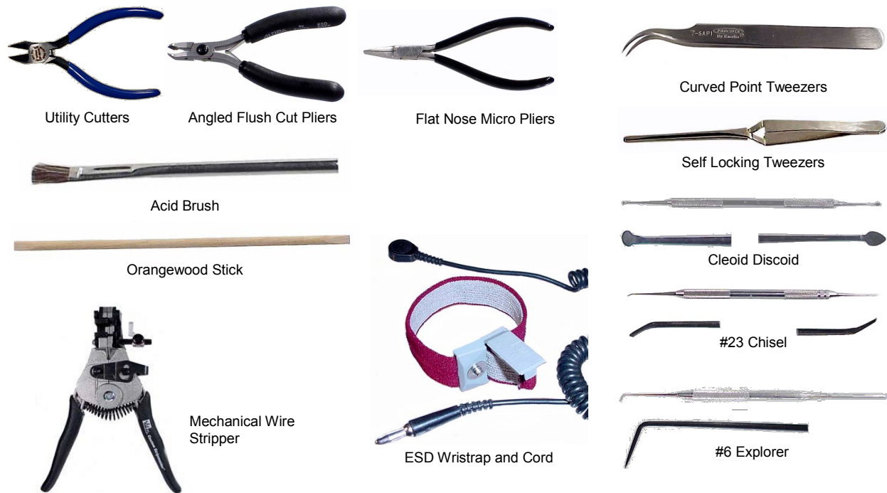
Figure 6.—Images of recommended hand and dental tools to allow for component-level repair of electronics. (Note that images are not to scale.)
