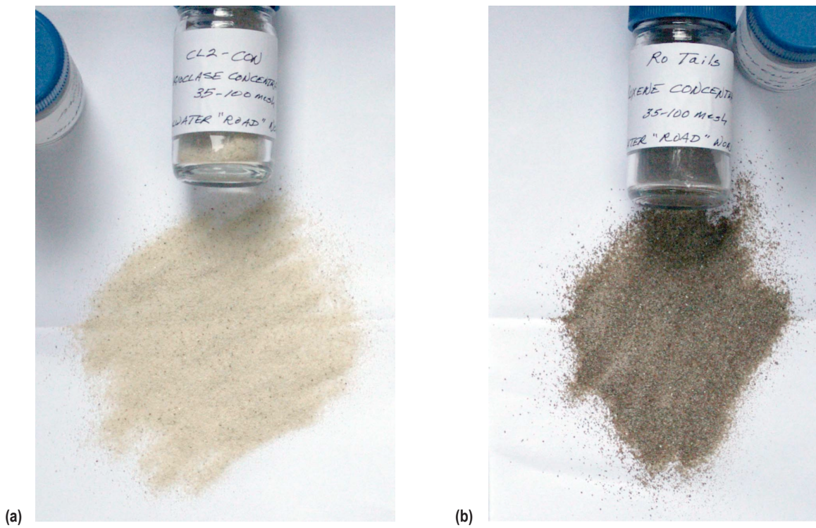
Figure 33. The concentrate 33(a) and tails 33(b) from the 35–100-mesh fraction as processed according to figure 31. The photo of the tails in figure 33(b) shows marked segregation of colors
