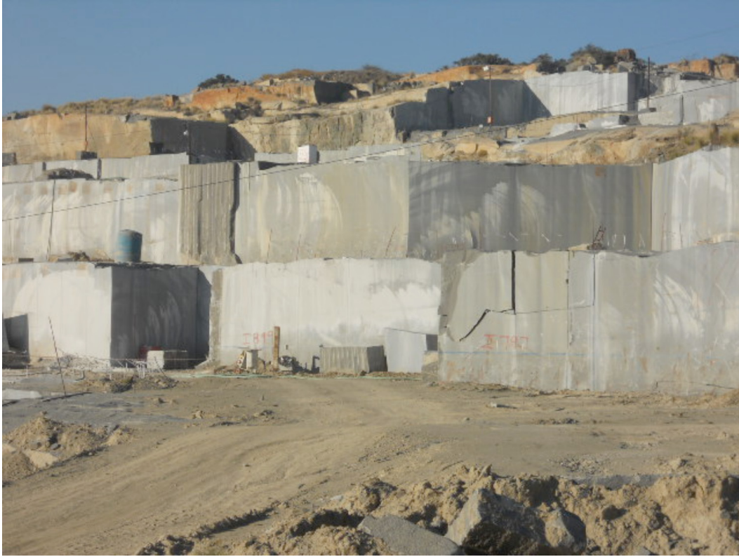
Figure 41. Working faces in quarry shown in figure 40. Almost all of the rock in view is functionally identical for the purposes of simulant utility. Image by Jonathan Houghton.
