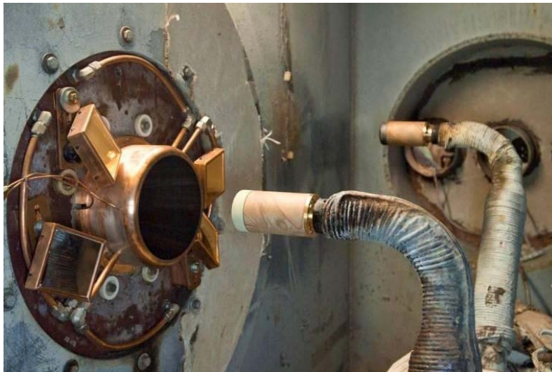
Figure F-4. Model Injection System Showing Two Sting Arms.
