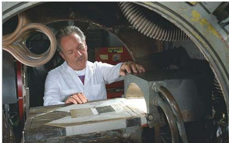
Figure F-14. Panel Test Facility Test Cabin showing Semi-Elliptic Nozzle and Test Panel.
