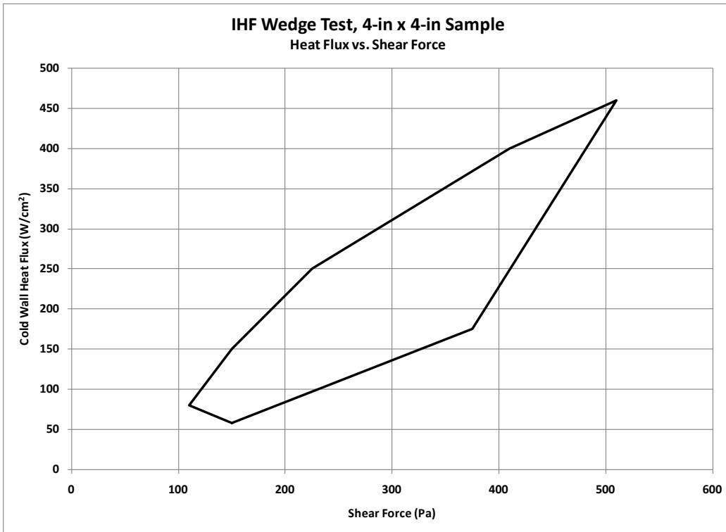
Figure F-8. IHF Wedge test Capability on a 4-in x 4-in Sample, Heat Flux vs. Shear Force.
