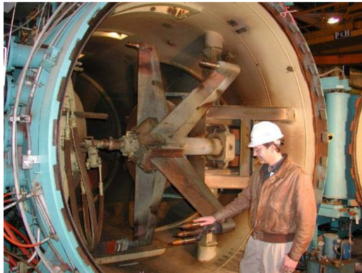
Figure F-26. View of AEDC H2 facility Test Cabin and Model Injection System.
