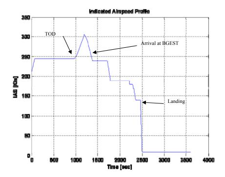
Figure 69 Indicated Airspeed Profile
