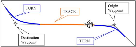
Figure 41 – Flight Segment and Navigation Modes
