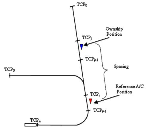
Figure 8 - Representative Layout of Paired Airplanes in Precision Spacing Mode
