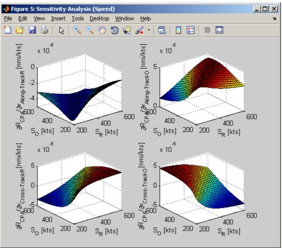
Figure 20 – TPS Sensitivity to Velocity Error as a Function of S<sub>0</sub> and S<sub>R</sub>.
