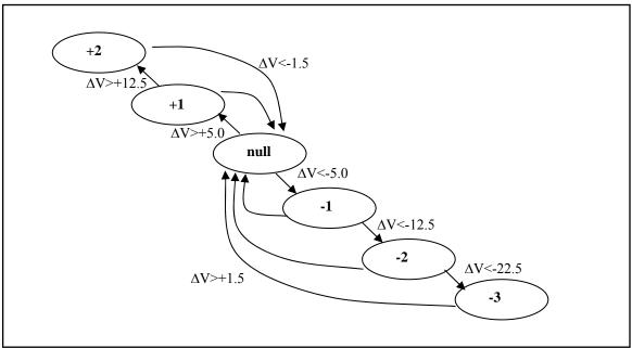
Figure 51 – Speed Change Logic
