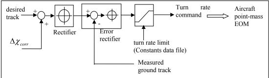
Figure 48 – Lateral Control System in TRACK mode
