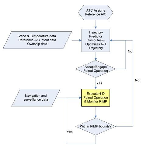
Figure 37 – RIMP Operation Flow Diagram
