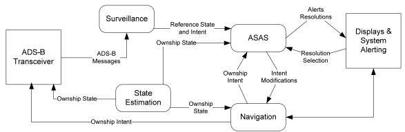
**Figure 1 - Separation System Functional Block Diagram**
