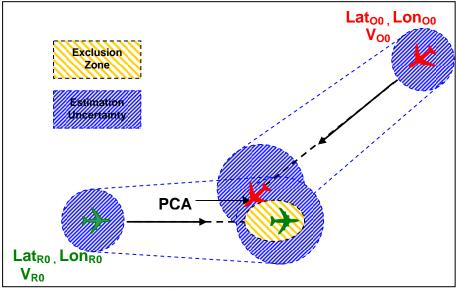
**Figure 5 - Estimated Geometry with Uncertainties and Errors**
