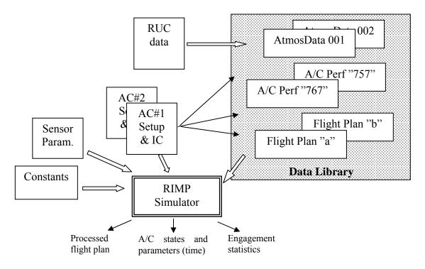
Figure 39 – RIMP model data flow
