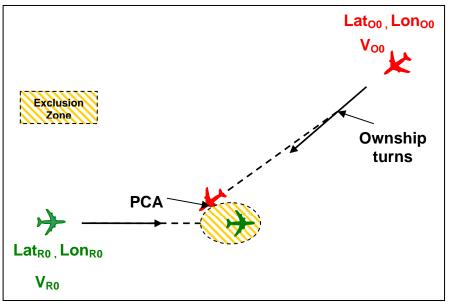
Figure 4 - Estimated Geometry after Ownship Turns
