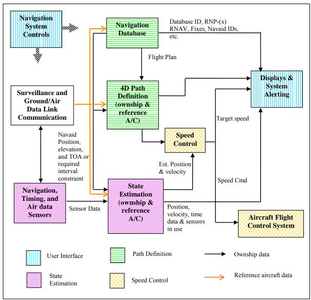
Figure 7 - APS System Block Diagram
