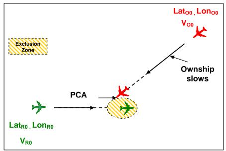
Figure 3 - Estimated Geometry after Ownship Slows
