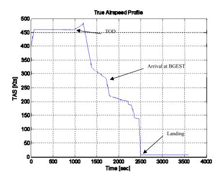
Figure 71 True Airspeed Profile
