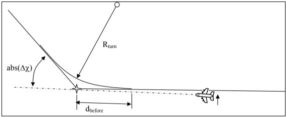
Figure 43 – Required Distance for Turn to New Course
