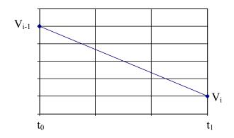
Figure 50 – Assumed velocity profile for descent segments
