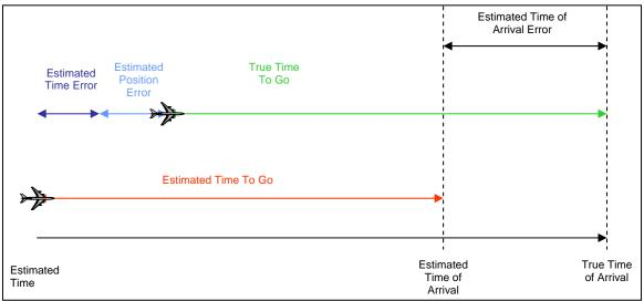
Figure 9 - Along Track Components of Navigation Error Terms
