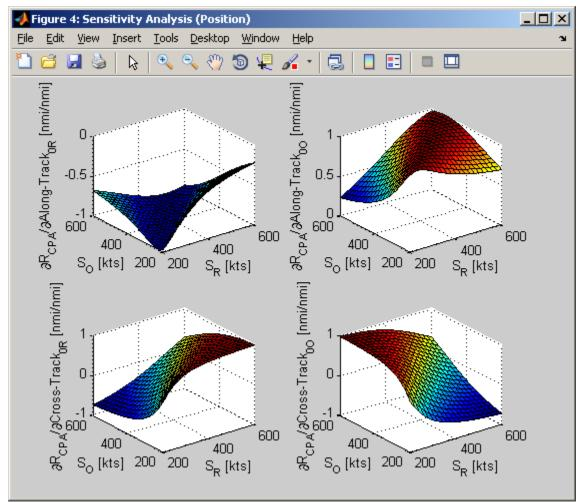
Figure 19 – TPS Sensitivity to Position Error as a Function of S<sub>0</sub> and S<sub>R</sub>.
