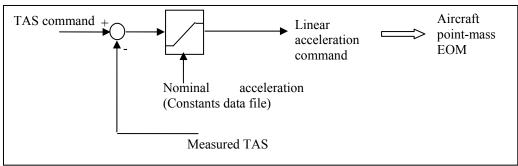
Figure 46 – True Airspeed Control System
