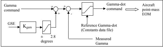
Figure 47 – Vertical Flight Path Control System
