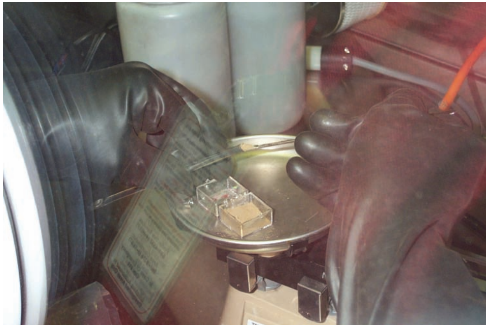
Figure 142. Simulant being loaded in Ar-filled glovebox. Note the box of simulant on the balance pan.
