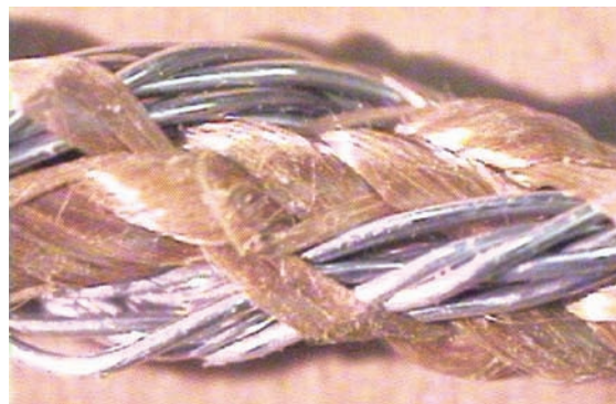
Figure 90. Eight 278 decitex ZYLON yarns, six 3270 decitex ZYLON yarns, and two Al wire braids braided together (1.4871 g/ft) creating the pseudocore braid.
