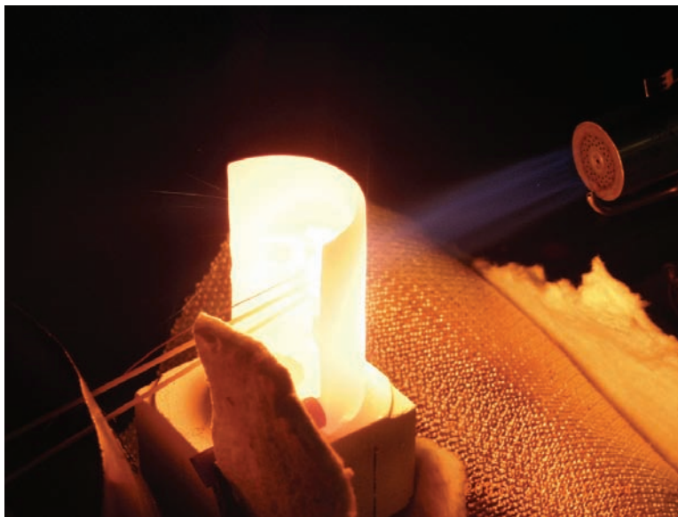
Figure 177. A close-up view of the test in figure 175 showing thermocouple placement. Two B-type and one K-type thermocouples were used.
