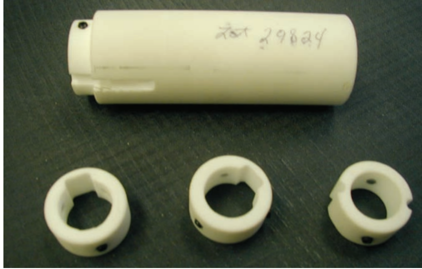
Figure 218. Macor end piece and spacers to locate the rod heater in the center of the Ti tube. The spacers are attached to the heater rod using the small-set screws. The inside notches accommodate the thermocouples that measure the heater temperature. The outside grooves allow passage of the thermocouple wires.
