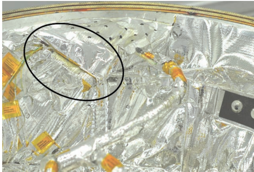
Figure 24. Contamination visible in normal light on backshell MLI; circled area is shown again in figure 25.
