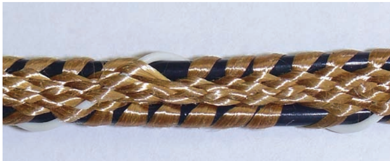
Figure 92. Sixteen 278 decitex ZYLON yarns in a braid with four 3270 decitex ZYLON yarns and two 16-AWG wires as axials.
