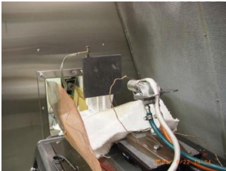
Figure 175. Plate of graphite under test with H-O torch. Longer target life was found, but no measurable bias influence. Likely very low plasma yield.
