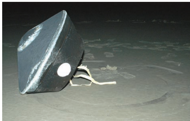
Figure 3. Stardust spacecraft immediately after landing at UTTR. Note the roll track in the dirt.
