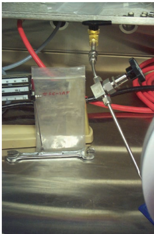
Figure 143. Inconel 625 tube after filling with lunar simulant. The tube is shown attached through a valve to the vacuum line. Arms from the balance are shown on the left.
