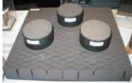
Figure 228. Solar tower test of ablator panel.
