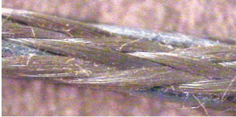
Figure 89. Fourteen 278 decitex ZYLON yarns and two Al wires braided together.
