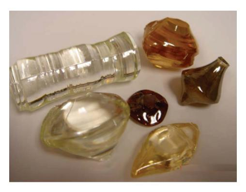
Figure 14. Pure and doped LN crystals grown at AAMU.
