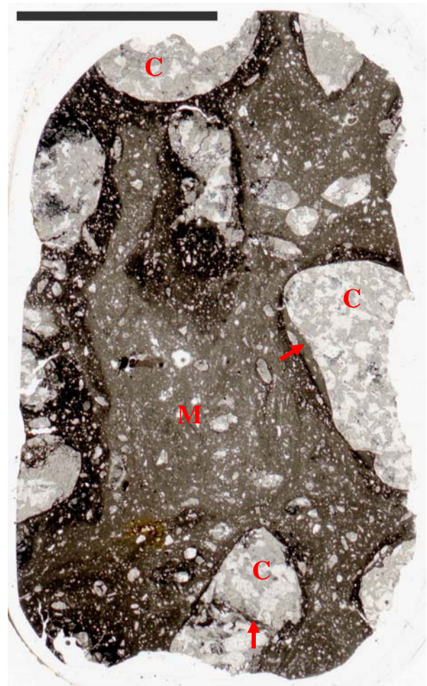
Figure 1. Thin section scan of NWA 5218. Black bar is 1 cm long. C - clast, M - melt; arrows indicate trachytic-textured melts.
