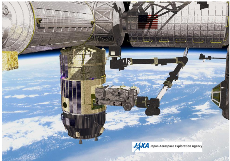
Figure 3. HTV berthed to the underside of Node 2. SSRMS is still attached to the HTV. The use of the robotic arm creates increased risk of collision.
