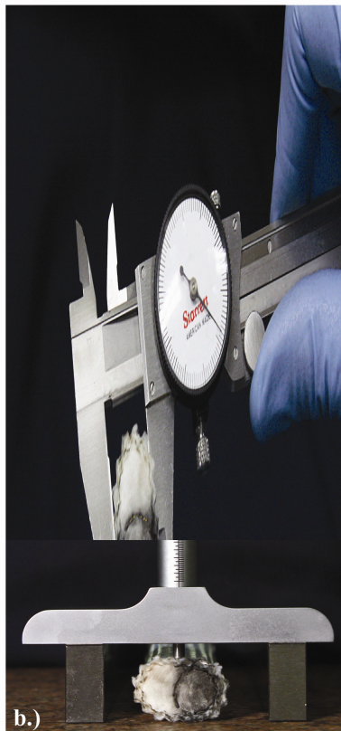
Figure 2.—Manual techniques classically used for thermal barrier measurement: a.) dial caliper, and b.) depth micrometer with precision parallels.
