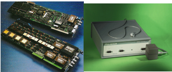
Figure 2. Left: Convolvotron card set. Right: Polhemus Isotrak head tracking hardware, including transmitter and receiver
