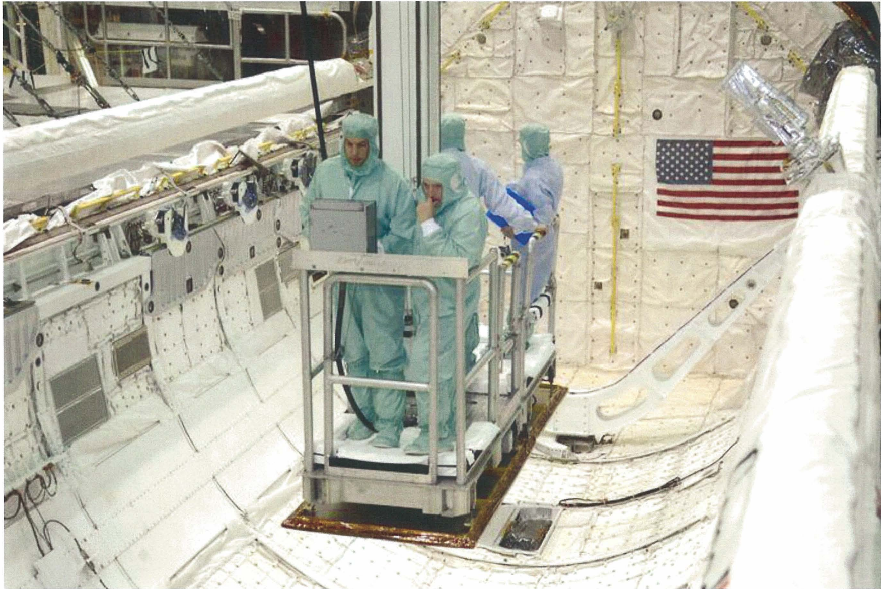
OPF Payload Bucket Hoist
