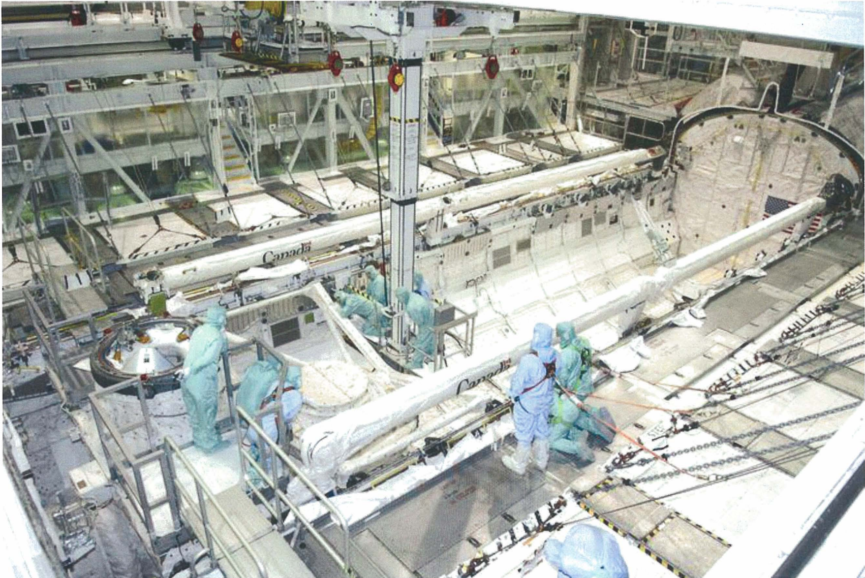
OPF Payload Bucket Hoist
