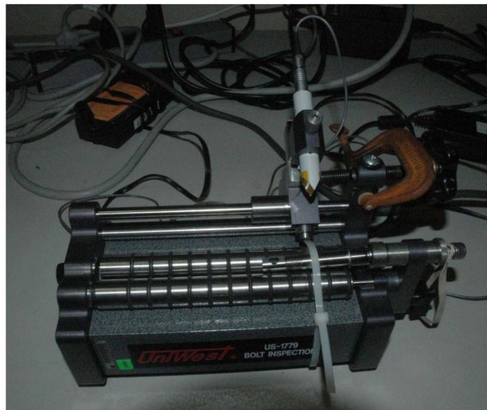
Figure 10: Poppet Positioned for Radius Scanning
