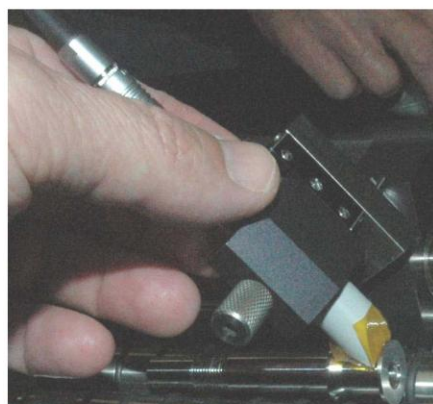
Figure 3: US-1839 Probe with "V" Shape 0.0312" Radius
