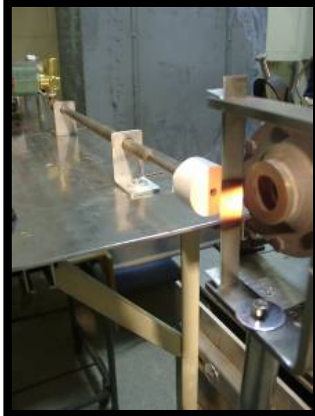
Figure 11.—Top: The small cylinder is filled with helium from the “K” bottle, and the “Red Hat” valve is actuated to accelerate the round projectile toward the sample down a hypodermic metal tube (1/16 in. ID) inserted in a larger diameter (1/8 in. ID) stainless steel barrel. Bottom: Business end of impact gun. Exit of barrel is protected from the flame with ceramic insulation. In this case, a superalloy target sample is held in a “C” clamp arrangement.
