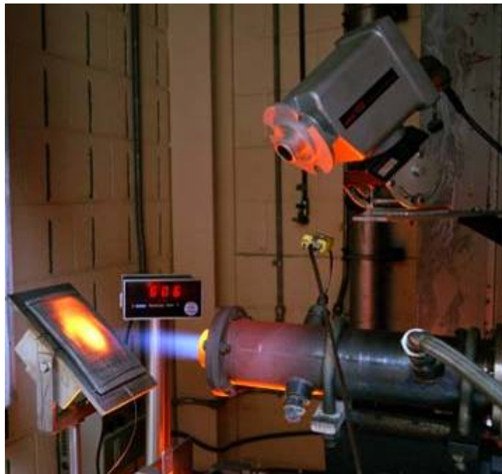
Figure 2.—Mach 0.3 burner used in thermal blanket durability study. (NASA photo C-1994-5005, November 1994, from Ref. 33).
