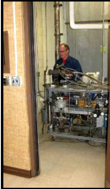
Figure 6.—Top: Mach 0.3 burner rig facility control room. Each of the seven rigs is housed in individual test cells behind the operator as he sits. Bottom: Looking through the soundproof door into one of the test cells.
