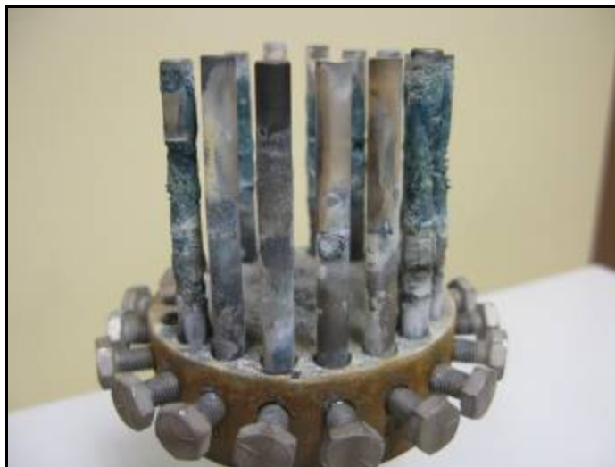
Figure 10.—Results of the above 900 °C (1650 °F), 500 hr corrosion test with 8 ppm synthetic sea salt. The most corrosion resistant samples are located at the forefront.
