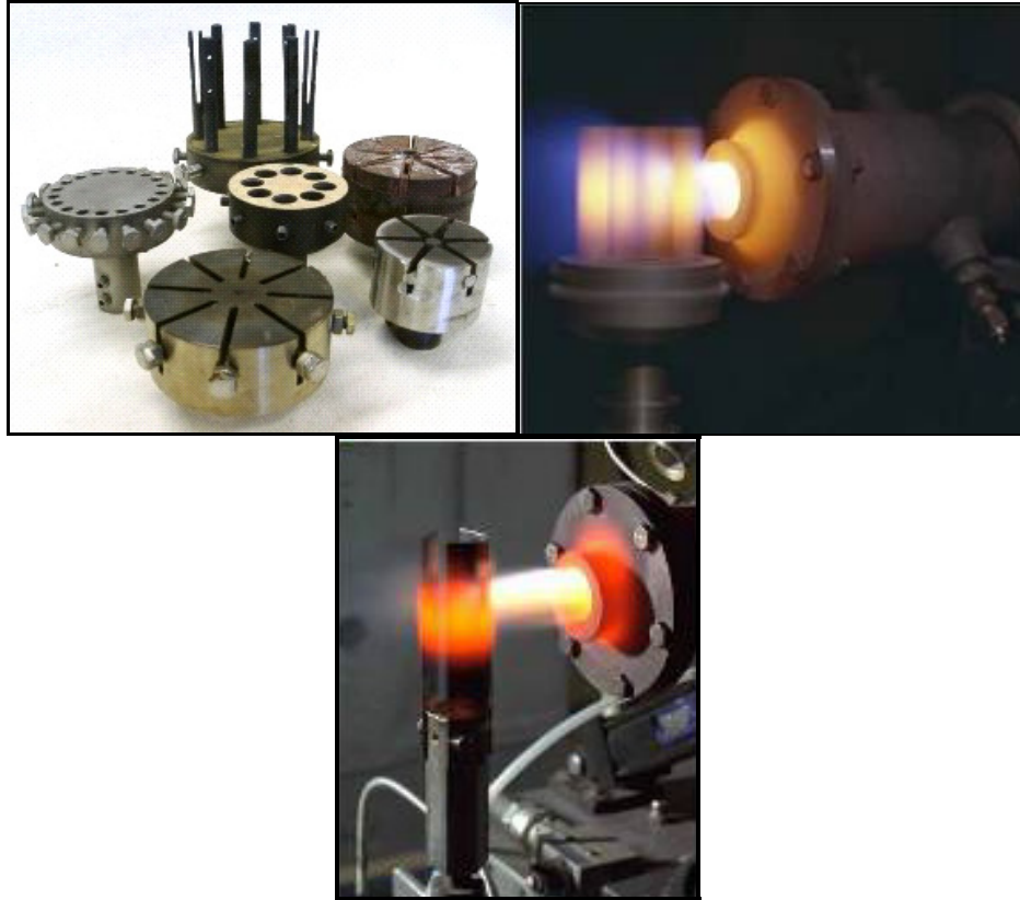
Figure 5.—Top left: Assortment of carousels used for cylindrical, rectangular, and occasional odd-shaped samples (such as those in Fig. 20). Top right: Cylindrical sintered \alpha -silicon carbide samples in test carousel (NASA GRC photo C-1991-10893). Bottom: Superalloy sheets in carousel test (C-1999-2482).
