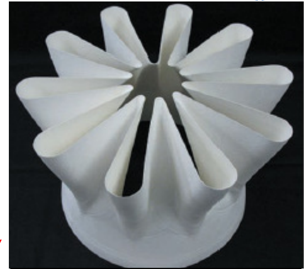
18-inch dia. CMC Mixer Demo article (ATK / COIC)
