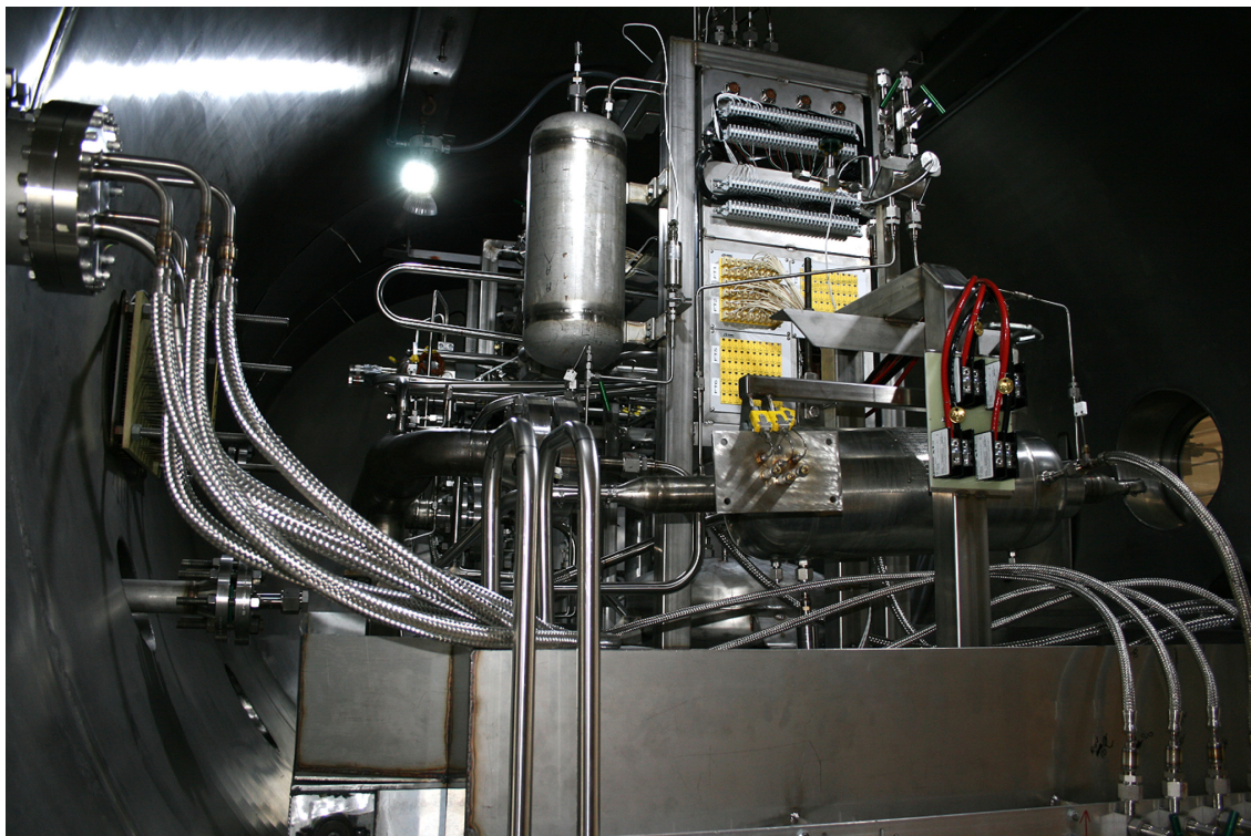
Figure 7.—FSP–PTC completed and installed into the vacuum chamber prior to insulation.
