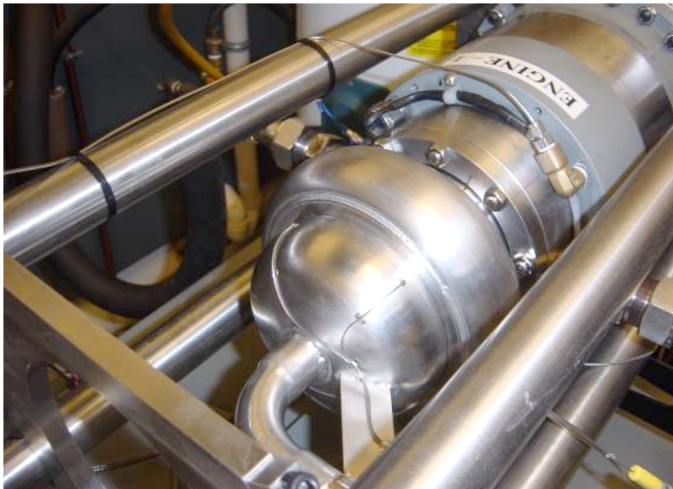
Figure 3.—Single P2A free-piston Stirling power convertor with NaK heat exchanger prior to installation of multilayer insulation (MLI).
