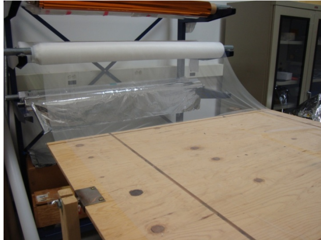
Figure 6. Rolling out Dacron B4A for cutting
