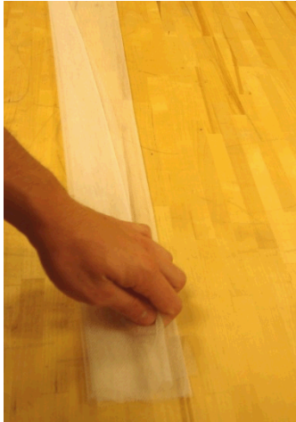
Figure 5. Folding bumper strips
