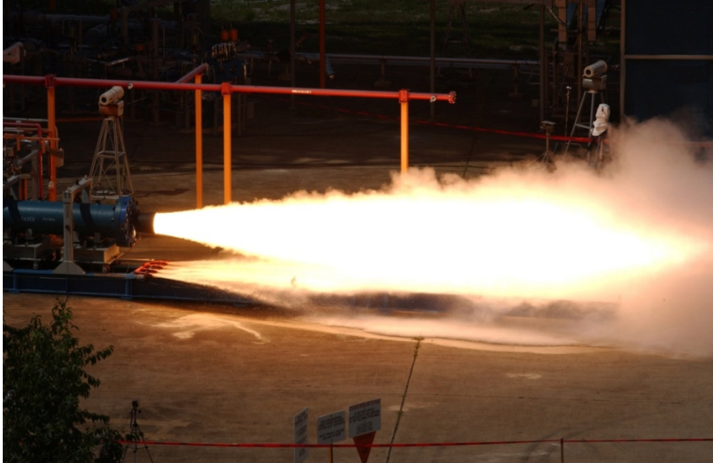
Figure 51. A Scaled-Down 24-Inch Version of the Space Shuttle's Reusable Solid Rocket Motor Fired at a MSFC Test Stand
