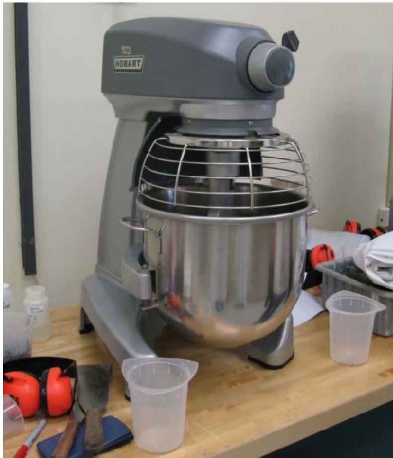
Figure 14. Paddle Mixer Used at KSC To Prepare Refractory Samples
