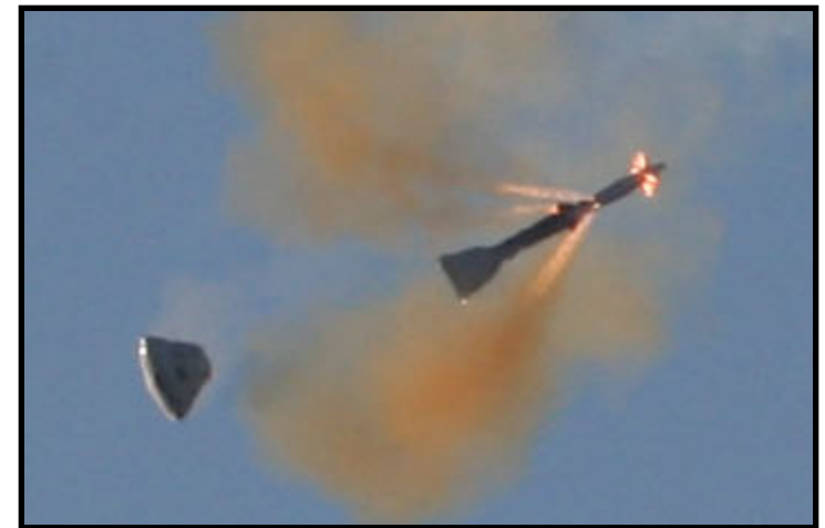
Picture showing orientation of Crew Module and Launch Abort System just after LAS jettison
