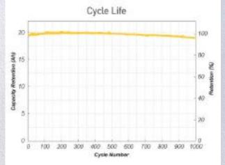
CHARGE : CC(1.0CI/CVI4.15V to 0.05Cl at 25°C DISCHARGE : CC(1.0C) to 3.0V at 25°C (DQD100%).
