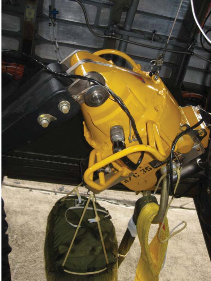
Figure 21. Programmer pack and risers attached to hook.
