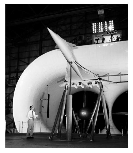
NASA research engineer Dave Hahne inspects a tenth-scale model of a Supersonic Transport model in the 30- by 60-foot tunnel at Langley. The model is being used in support of NASA's High Speed Research program. (NASA Langley Research Center [NASA LaRC].)
