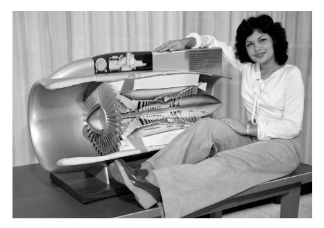
Model of the  $E^3$  technology improvements. These included improved component aerodynamics, improved compressor loading, active clearance control, low emissions combustor, and higher-temperature materials. (NASA Glenn Research Center [NASA GRC].)
