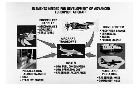
Advanced Turboprop elements, including the propeller, nacelle, aerodynamics, and noise control. (NASA Glenn Research Center [NASA GRC].)
