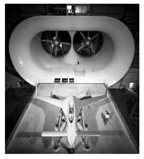
Composites technology was applied to other projects as well. The Rutan Model 33 VariEze was built by the Model and Composites Section of Langley and then tested in a tunnel. (July 17, 1981). (NASA Headquarters—Greatest Images of NASA [NASA HQ GRIN].)
