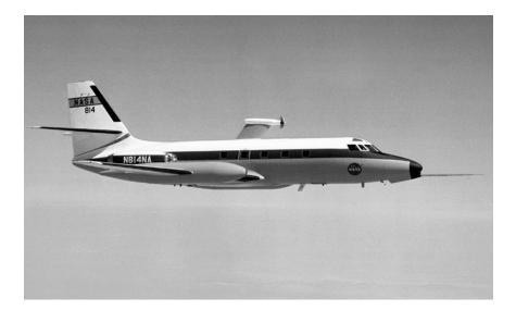
The Dryden C-140 JetStar during testing of advanced propfan designs. Dryden conducted flight research in 1981–1982. The Lewis Research Center directed the technology's development under the Advanced Turboprop program. Langley oversaw work on acoustics and noise reduction. The effort was intended to develop a high-speed, fuel-efficient turboprop system. (January 1, 1981.) (NASA Dryden Flight Research Center [NASA DFRC].)
