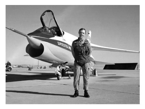
NASA selected a Vought F-8A Crusader as the testbed for an experimental supercritical wing. (January 1, 1972). (NASA Dryden Flight Research Center [NASA DFRC] Photo Collection.)
