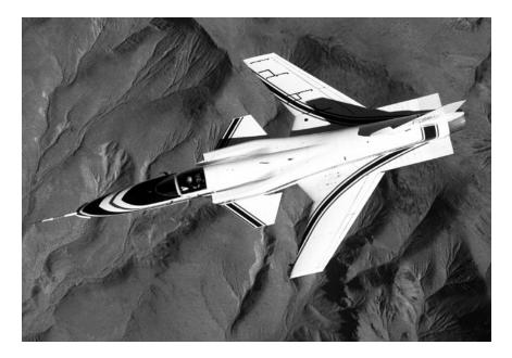
This X-29 research aircraft in flight over California's Mojave Desert shows its striking forwardswept wing and canard design. The X-29 demonstrated the use of advanced composites in aircraft construction. Two X-29 aircraft flew at the Ames-Dryden Flight Research Facility from 1984 to 1992. (NASA Dryden Flight Research Center Photo Collection.)
