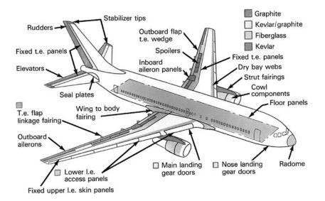
The above graphic demonstrates the composite components of the Boeing 767. Courtesy of Joseph Chambers.
