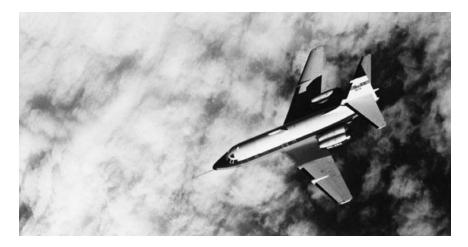
Laminar flow test aircraft in flight (November 15, 1984). (NASA Langley Research Center [NASA LaRC].)
