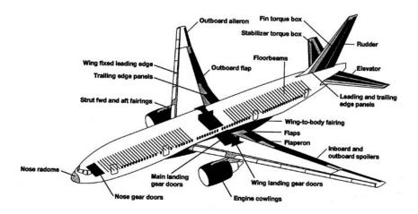
The above graphic demonstrates the composite components of the Boeing 777. Courtesy of Joseph Chambers.
