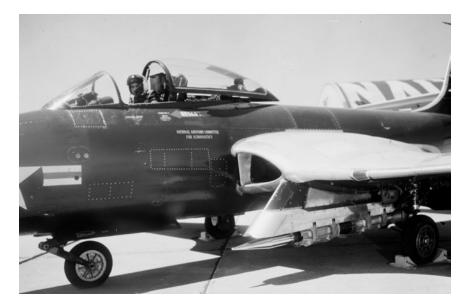
Early laminar flow tests on a blunted 15-degree cone cylinder in free flight at high Reynolds number (July 23, 1956). (NASA Glenn Research Center [NASA GRC].)
