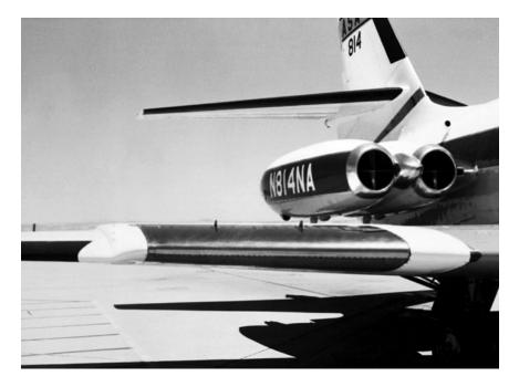
The center section of each wing of this business jet was modified for tests of laminar flow control (October 15, 1984). (NASA Langley Research Center [NASA LaRC].)
