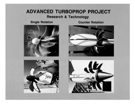
Single- and counter-rotation turboprops. (NASA Glenn Research Center [NASA GRC].)
