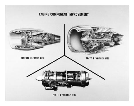
Three of the engines studied in the Engine Component Improvement (ECI) project. The ECI engineers' mission was to improve various components on existing engines that were most likely to wear and decrease fuel efficiency. (NASA Glenn Research Center [NASA GRC].)
