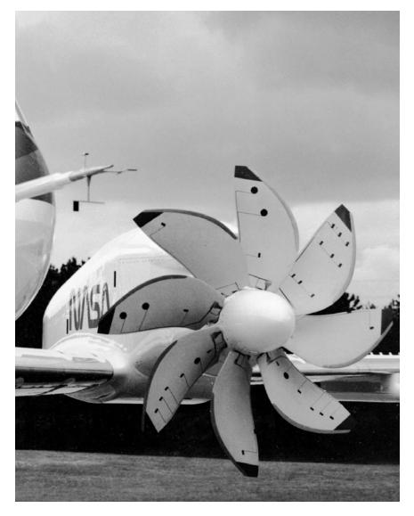
SR-7L Advanced Turboprop on gulfstream jet in 1987. (NASA Glenn Research Center.)
