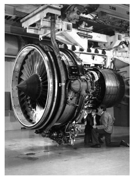
GE Energy Efficient Engine (June 16, 1983). (NASA Glenn Research Center [NASA GRC].)
