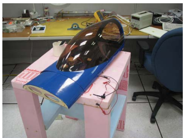
Figure 11: Laboratory Use of Non-magnetic Level Table for Hard/Soft Iron Compensation of AHRS Magnetic Reference Vector
