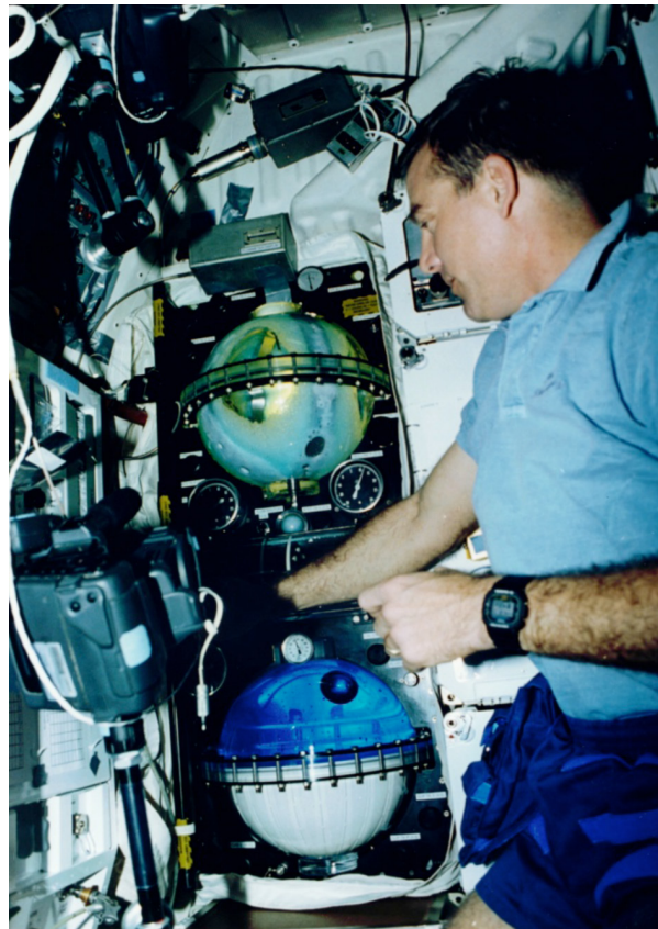
Figure 13. Overview of liquid condition during evacuated tank screen channel tank fill.
