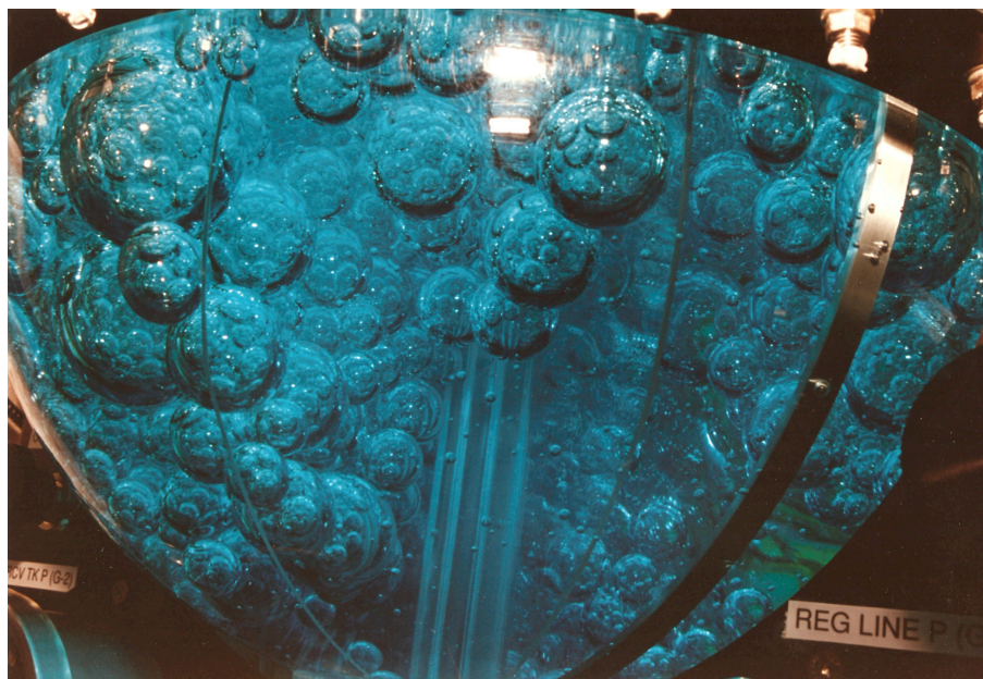
Figure 25. Vane tank expulsion with high bubble density.
