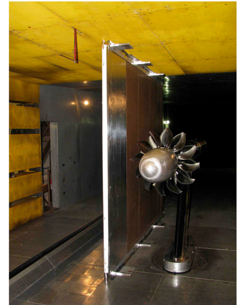
Semi-infinite acoustic barrier wall.
