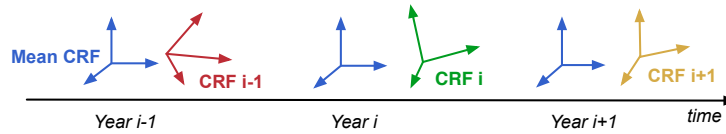
Figure 1. Stability test scheme. This figure illustrates the method used to judge the stability of a subset of sources by comparing yearly averaged Celestial Reference Frames (CRF)_i to a mean CRF.
