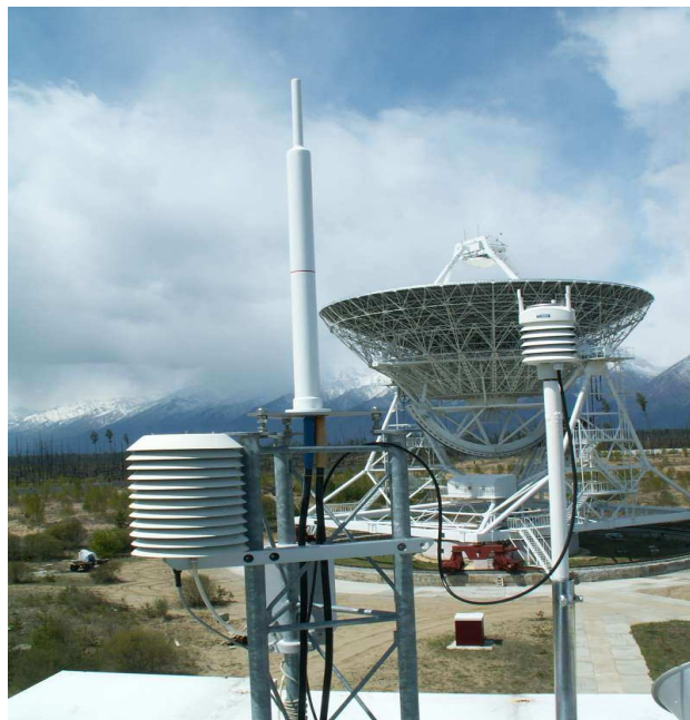
Figure 1. Badary's DORIS Starec-type antenna and RT-32 radio telescope. View from control block.
