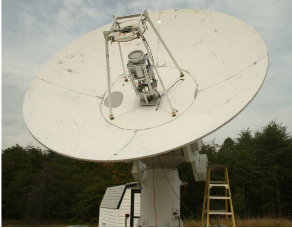
Figure 2. MV-3 5-m antenna at GGAO with the VLBI2010 proof-of-concept Dewar mounted at the Cassegrain focus.
