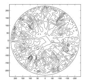
Figure 1. Contour map showing the deviation of the measured main reflector surface from the theoretical one. Ten contours are used in the range from -0.5 to 0.5 mm. X and Y axes are in inches.
