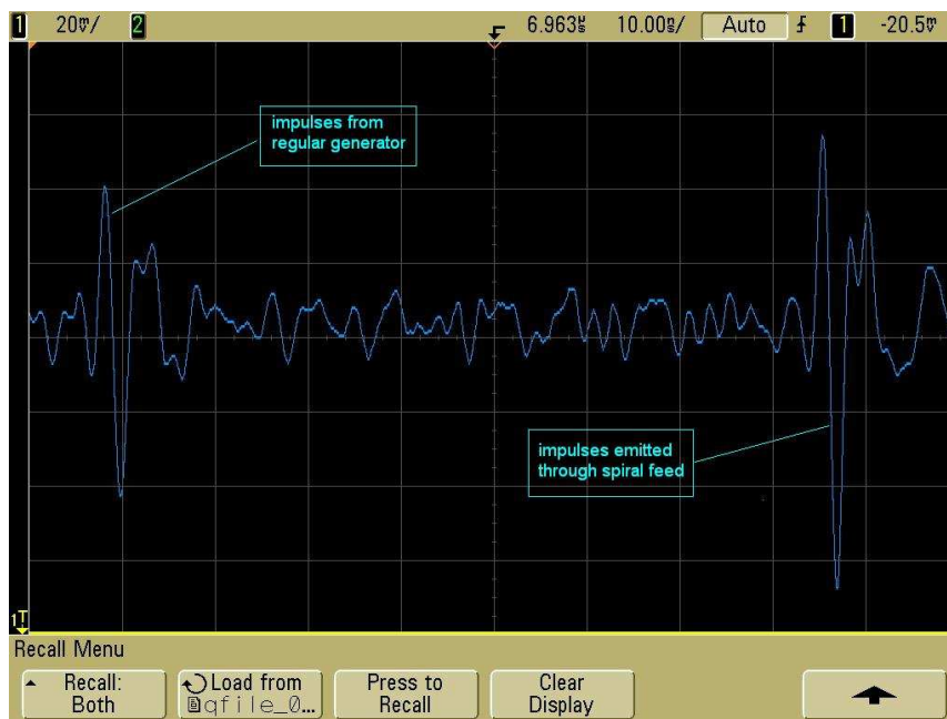
Figure 4. Oscillogram of the output signal from the S-band receiver.
