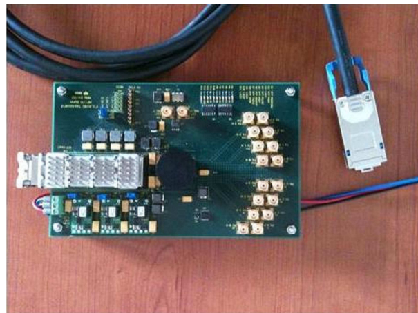
Figure 2. GLAPPER (glass to copper) prototype board to connect a DBBC with a Mark 5C.
