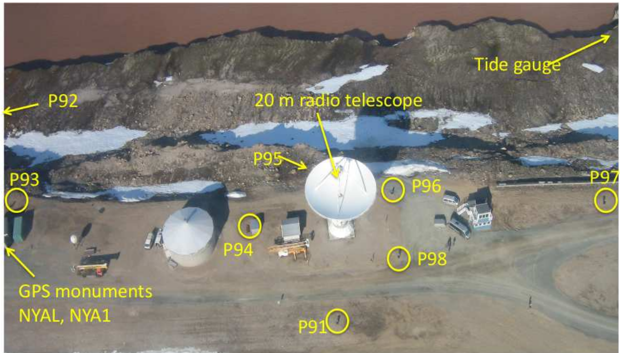
Figure 1. Aerial picture of the Geodetic Observatory Ny-Ålesund on Svalbard. The VLBI telescope and GNSS monuments and some of the survey pillars of the local survey network are depicted.
