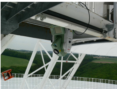
Figure 3. Leica TCRP 1201, mounted top-down.
