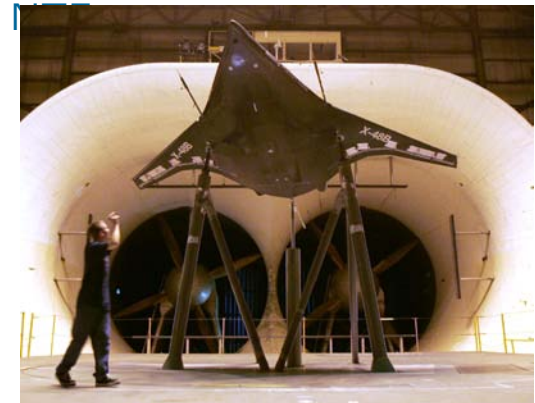
X-48B strut mounted in Langley Full Scale Tunnel
