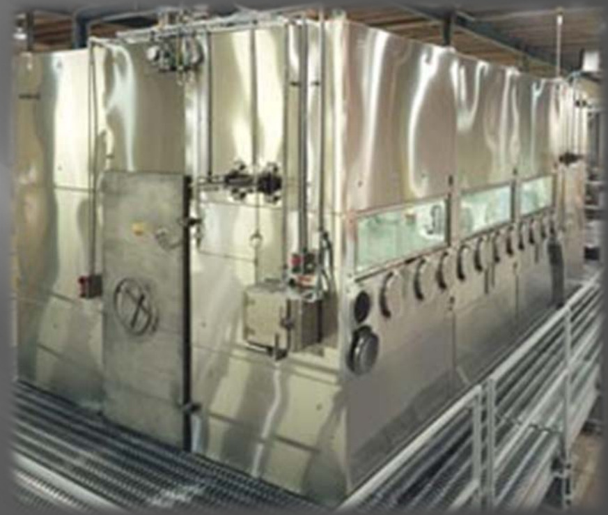
IP Systems Cold Testing Glovebox/Chamber - 40 °C, Class 100 environment
