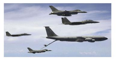
Aerial Refueling: The process of transferring fuel from one aircraft (a tanker) to another (a fighter as a receiver) during flight.
