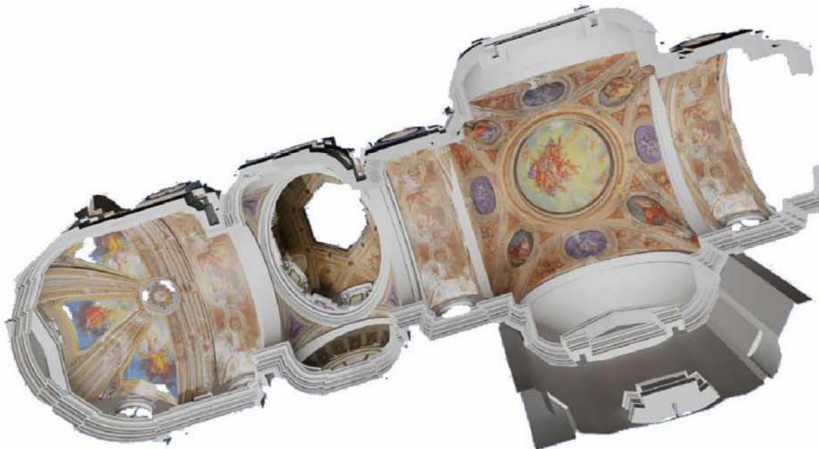
3D model based on architectural surveys in scale 1:50 performed by the team of Department of Building Engineering and Territorial Systems and Department of Land, Environment and Geo-Engineering.
