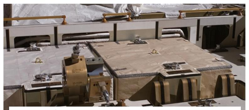
Battery Box Covers have a "Betacloth" outer layer. One cover was inadvertently constructed using Chemfab 250 (with silicone sizing agent not removed during its fabrication) while other cover was correctly constructed using Chemfab 500.
