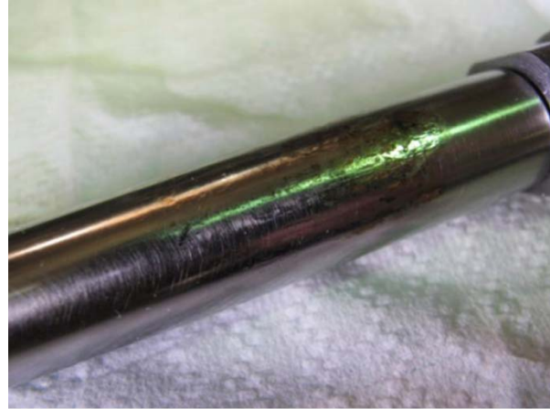
Figure 7.—Minor fretting on loading arm.
