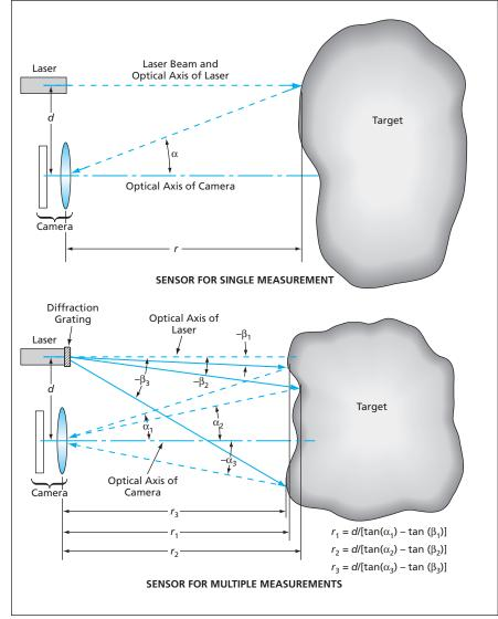
These **Two Sensors** would utilize triangulation to measure ranges. The simpler sensor is shown at the top, mainly to help explain the basic principle of operation. The more complex sensor shown at the bottom would likely be preferable in practice.
