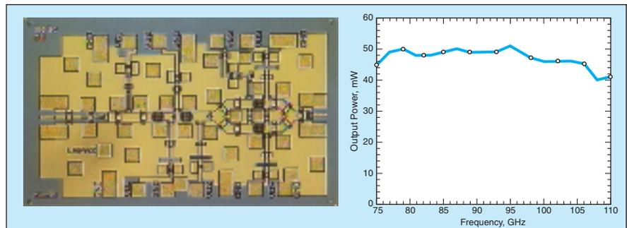
The Amplifier Shown in the Photograph was tested at a supply potential of 2.5 V, a gate bias potential of  $-0.05$  V, and an input excitation power of 2 mW at frequencies from 75 to 110 GHz. The plot of output power vs. frequency can be characterized by a large-signal gain of about  $13.5 \pm 0.5$  dB. (Note: The amplifier is actually about 2 mm long.)
