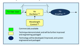
Figure 1: Block diagram of proposed  $2\mu m$  laser transmitter, illustrates the focus of the development approach
