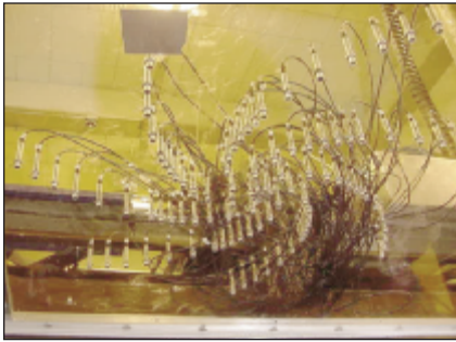
Figure 1. The Array of Microphones was mounted above the aircraft model in the test section of the wind tunnel. A cloth cover has been removed from under the microphones to make the model visible in this view.
