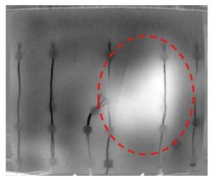
Figure 24. Thermography Image of IML showing delamination indicated by region within the dashed oval
