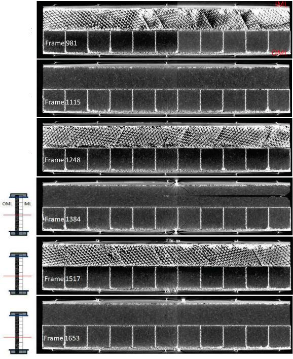
Note: Voids along intersection of overwrap and lower AETB bars Variation in porosity along OML (S200H)
