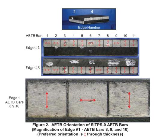
Prior to mechanical testing, the SITPS-0 test article was subjected to thermal testing.<sup>(2)</sup> The thermal testing required that several thermocouples be inserted into the AETB-16 material which resulted in gouges in the AETB-16 shown in Figures 2 and 3 (Figure 3 designated by  $\circ$ ). The white residue on the overwraps and the OML in Figures 2 and 3 is residue from glue that held the thermocouple wires in place.
