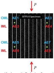
Figure 10. Acoustic Emission Sensor Location
