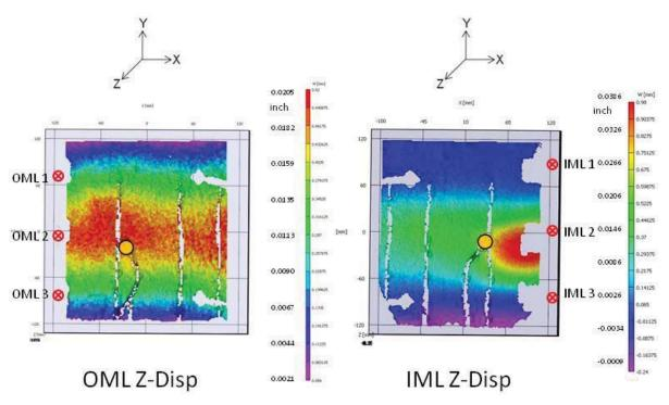
Figure 20. Out-of-Plane Displacements at P = 37K lbs (Photogrammetry System)
