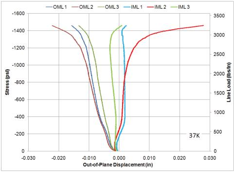
Figure 18. Out-of-Plane Displacements (DCDT) – 37K Loading Sequence
