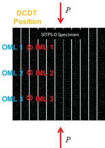
Figure 7. DCDT Layout for Bending and Out-of-Plane Displacements
