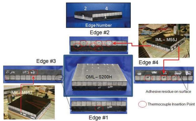
Figure 3. Surface Anomalies from Applied Instrumentation for Thermal Testing
