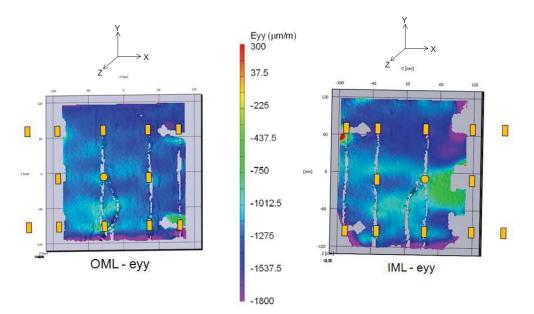
Figure 23. In-Plane Strains at P = 37K lbs (Photogrammetry System)
