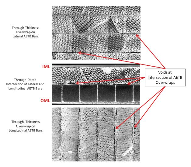
Figure B-2. Voids at AETB Overwrap Intersections
