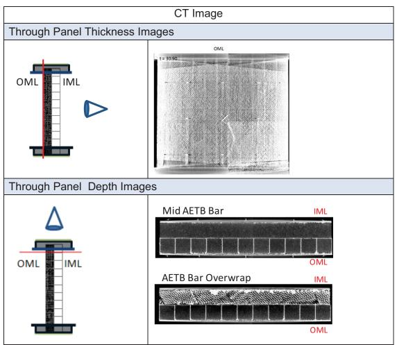
Figure B-1. Viewing Orientation for CT Images
