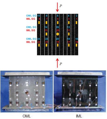
Figure 8. Strain Gage Locations for In-Plane Strains
