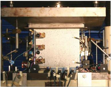
Figure 5. Instrumented SITPS-0 test article in test load frame (View of OML Facesheet)
