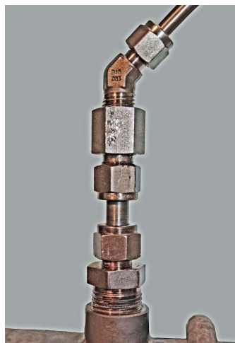
Figure 13.—Photograph of particle injector employing a 45° fitting.
